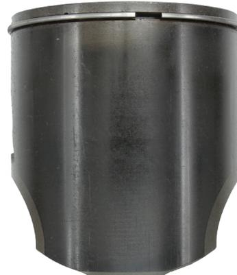
• PAS DE GRIPPAGE DES SEGMENTS DE PISTON • PAS DE FROTTEMENT DU PISTON
